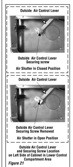
Operate the actuator through several cycles including the closed position. Ensuring proper operation and freedom of movement. Return the actuator arm to the closed position.
